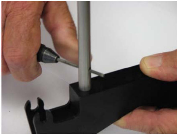
Ensure posts are tightly secured on brackets
