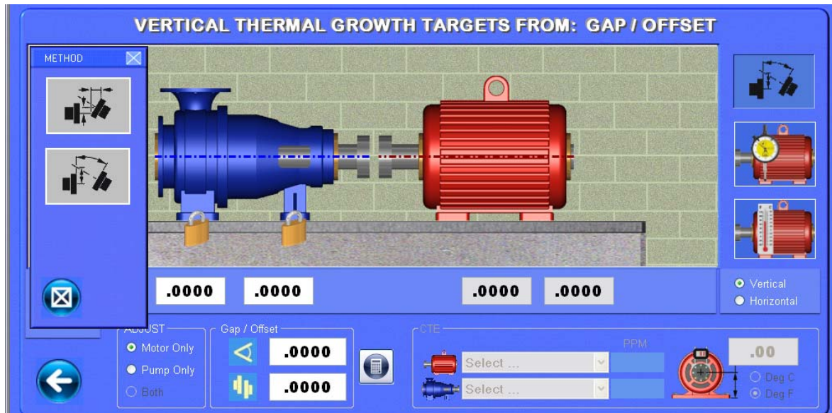
Figure 26 – Step 1: Thermal Growth at the coupling
