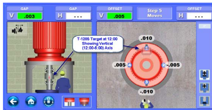
Figure 61 – Step 5: Vertical Pump Move Screen using the T-1285 Target at 12:00, showing Vertical Axis
