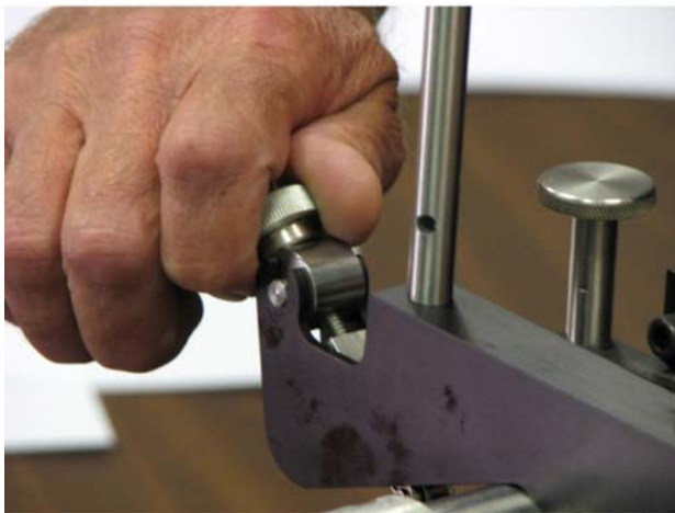
Tighten knob and fold chain (see 2B and 2C on Page 22)
