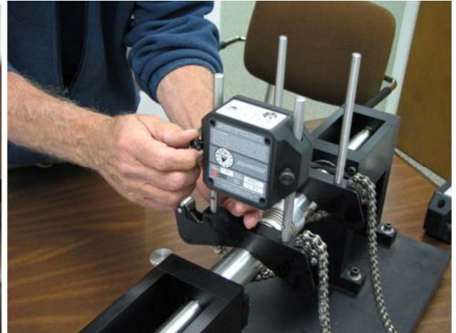
Slide target on A-970 bracket
