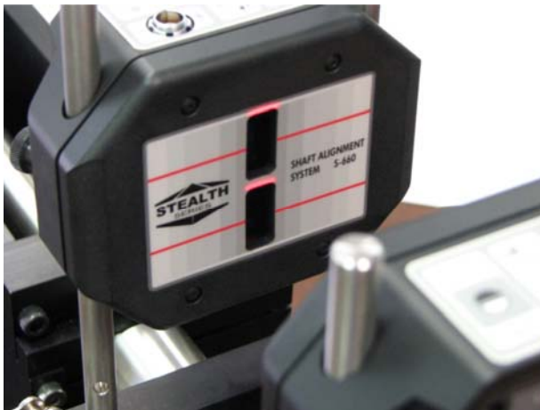
Adjust target height to center laser lines
