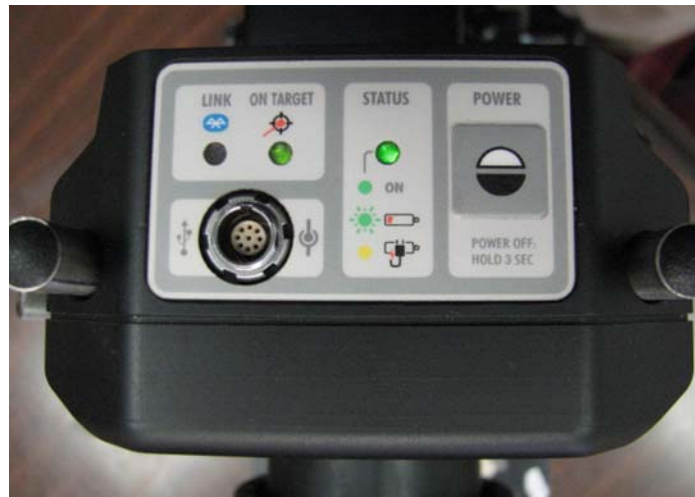
Figure 5 – T-1280 3-Axis Wireless Target (Top View)
