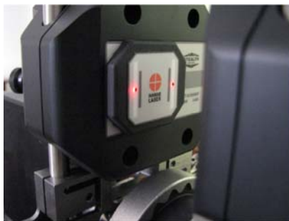
Figure 41 -- Aligning laser beams with S-670 to take uncoupled shaft data in Point Mode using the dust cover/alignment tool.
