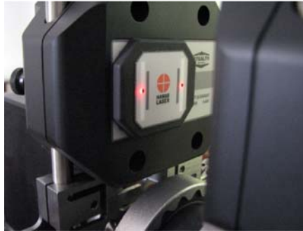
Figure 51 – Aligning laser beams with S-670 to take Uncoupled Shaft data in Point Mode using the dust cover/alignment tool
