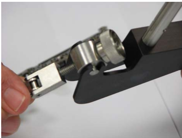
Attach chain to A-970 bracket (2)
