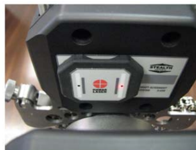
Figure 41 -- Aligning laser beams with S-670 to take uncoupled shaft data in Point Mode using the dust cover/alignment tool.
