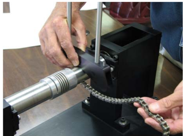
Wrap chain around the shaft
