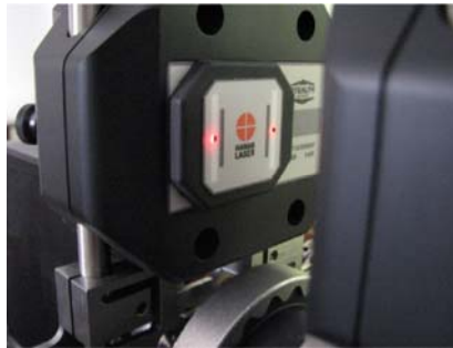
Figure 48 -- Aligning laser beams with S-670 to take Uncoupled Shaft data in Point Mode using the dust cover/alignment tool.
