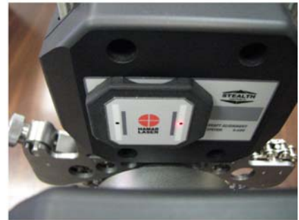
Figure 51 – Aligning laser beams with S-670 to take Uncoupled Shaft data in Point Mode using the dust cover/alignment tool
