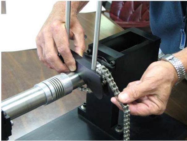
Attach chain to pin on A-970 bracket
