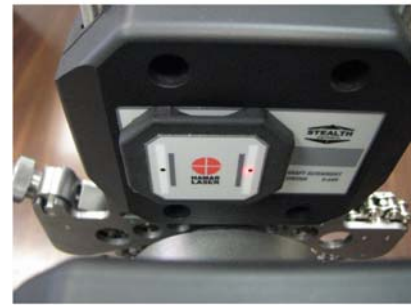
Figure 48 -- Aligning laser beams with S-670 to take Uncoupled Shaft data in Point Mode using the dust cover/alignment tool.
